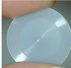
Figure 2.2.26: Fresnel lens (Reprinted from Wikipedia under the GNU Free Documentation License)
