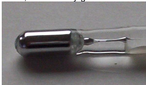
Figure 2.2.1: Mercury glass thermometer (Reprinted from Wikipedia under the GNU Free Documentation License)
