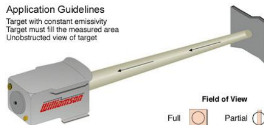
Figure 2.2.21: single wavelength sensor (Reprinted from Williamson's Free Specification Document)
