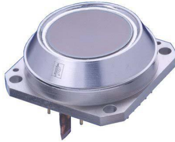
Figure 2.2.18: metallic package (Reprinted from Wikipedia under the GNU Free Documentation License)
